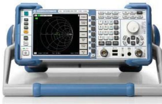
Figura 3-2: R&S ZVL Vector Network Analyzer [13].
