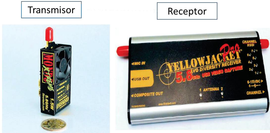
Figura 2-2: Transmisor Iftron Mondo Xtream 1.5 [W] [11], Receptor Iftron Yellow Jacket 5.8 [GHz] Pro [12].
