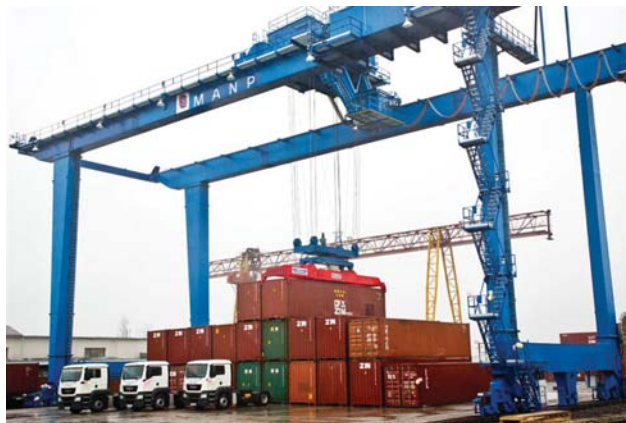
Figura 12: Rail Mounted Gantry Crane. Fuente: portstrategy.com
