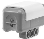
Figura 18 Sensor de Luz [LegoImag, 2001]
