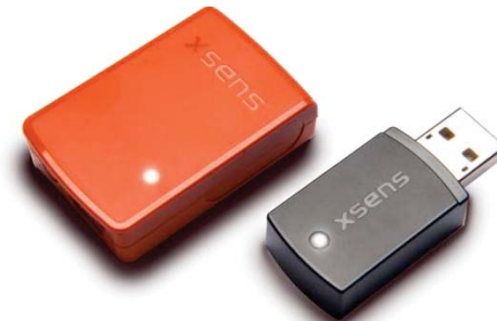
Figura 5-1: The Xsens MTw Awinda hardware y MTw Sensor; Awinda dongle (USB) (tamaño 47[mm] x 30[mm] x 13[mm], peso 16 [g]) [33].
