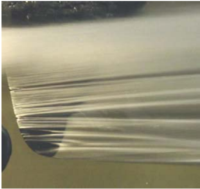
Figura 278. Ventilation on the back of the hydrofoil in model tests with free surface, same cavitation index of top speed. Fuente: Brizzolara, Bovio, Federici y Vernengo, 2011. Hydrodynamic Design of a Family of Hybrid SWATH Unmanned Surface Vehicles. 11th International Conference on Fast Sea Transportation, FAST 2011, Honolulu, Hawaii, USA.
