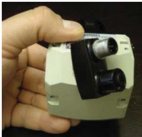
Figura 2-10 Sensor Sick Tim 551 (fuente: http://robotsforroboticists.com )
