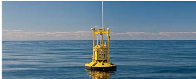
Figura 2-8 PowerBuoy PB150, UK. Potencia nominal 150 kW [25].
