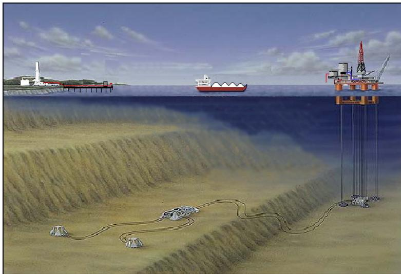
Figure 2.1478: Diagram to production of gas using ships to transport
