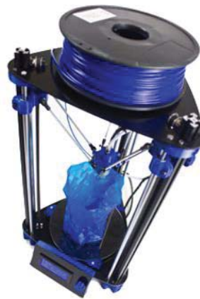
Figura 2-3:Impresora 3D, BCN Delta [11].
