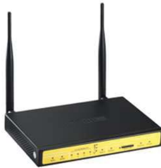
Figura 2-16: Router industrial Four-Faith. (Fuente: Four-Faith)
