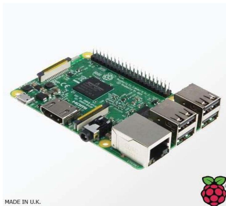
Figura 2-8 Raspberry Pi 3 model B.
