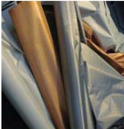
Figura 3-2: Material Conductor. Shieldex® Nora Dell. (Fuente: *Technical Textiles Inc., Technical Data Sheet, Shieldex® Nora Dell*).
