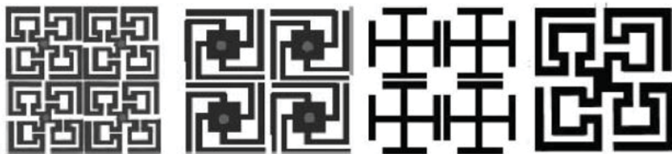
Figure 1.7: Several self-resonant grid structures. [61]
