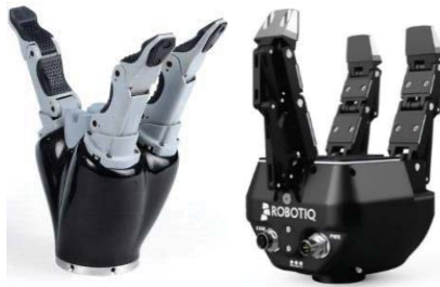
Figura 1-10: Pinzas de agarre Kinova KG-3 [24] y 3-Finger Adaptive Robot Gripper [27]
