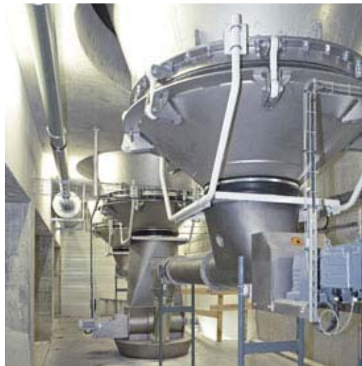
Fig. 17: MFVH Vibro extractor
